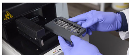
Multiple vial-holder being loaded into the ASA (Auto Sampling Array) accessory for measurement.
