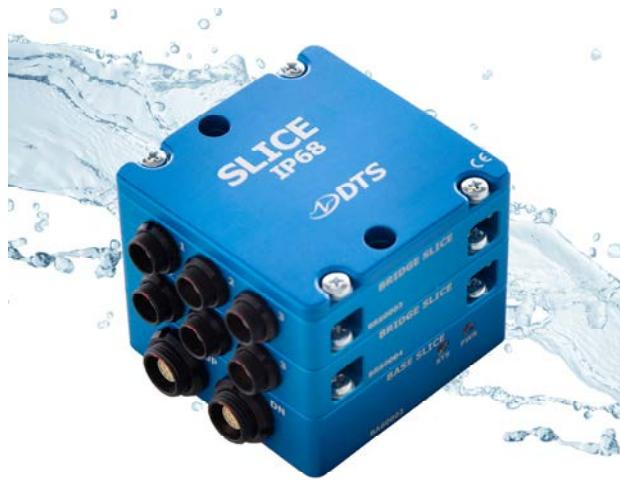
Designed for harsh test environments, the SLICE IP68 data acquisition system features IP68-rated connectors and enclosures. SLICE IP68 is modular and supports a variety of external sensors to measure acceleration, strain, voltage, temperature, plus offers layers with built-in sensor options.
