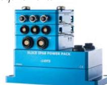
SLICE IP68 is a modular data acquisition system featuring unparalleled flexibility and reliability for extreme test environments. SLICE IP68 makes it easy to build systems in 3-channel increments by stacking layers with different sensor input configurations. The BASE+ is the foundation of the system with the microprocessor, memory and control circuits. A simple interface provides power, trigger, and communication signals. Data writes directly to non-volatile flash memory.
