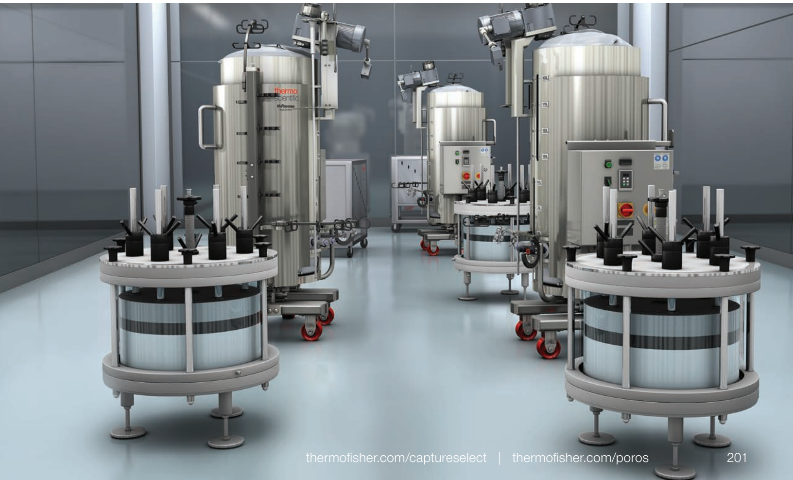
Figure 1. This workflow is depicting a typical downstream process for bio-therapeutics development. CaptureSelect and POROS resins can be used for both capture and polishing purification steps.
