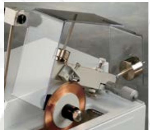
The optional Splash Guard Kit (11-1199) prevents coolant from spraying.
