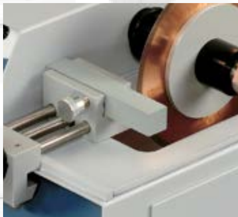
The optional dressing chuck (11-1196) allows dressing of the wafering blade without interrupting the sectioning process.
