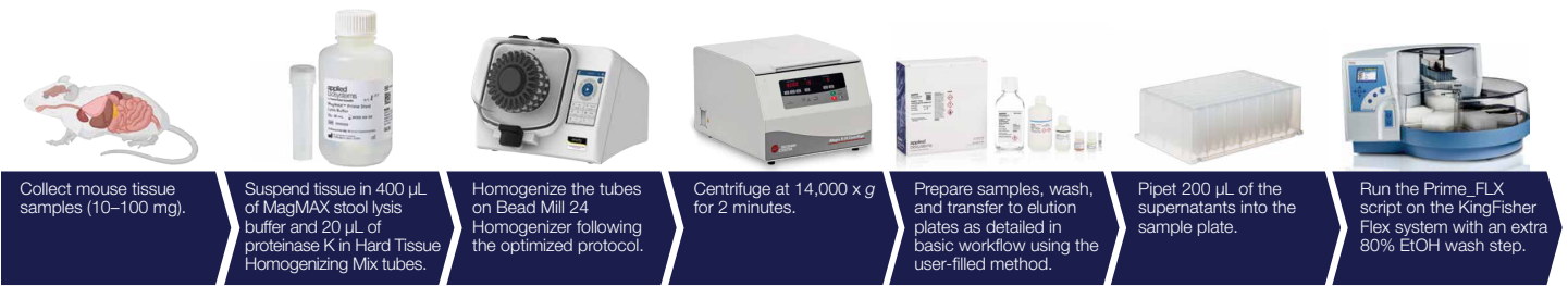
Figure 1. Overview of steps for extracting nucleic acid from tissue samples.
