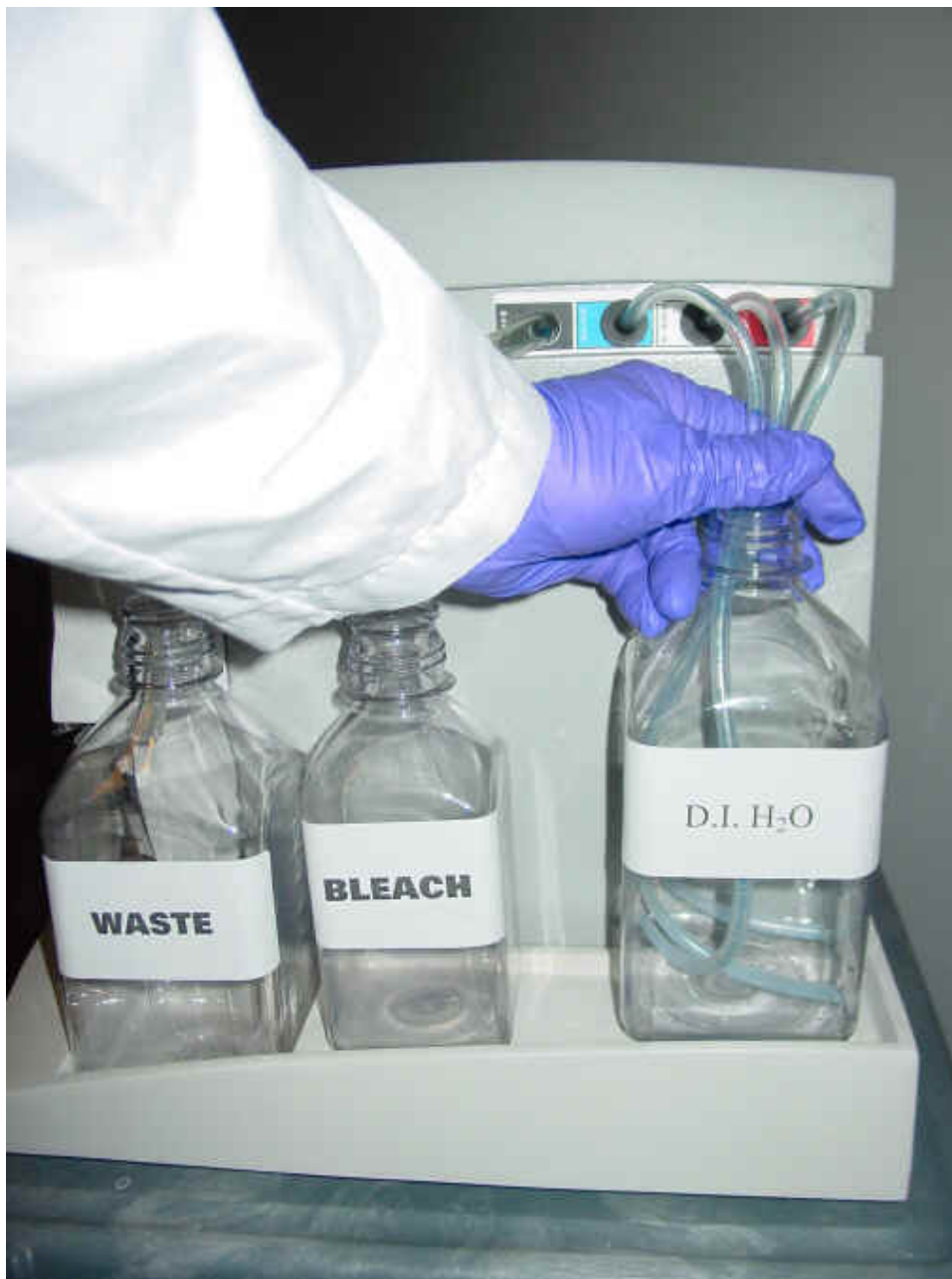
Figure 33 Immerse the three wash and water lines in the DI water bottle. At this step, there is no need to be concerned about the bleach remaining in the lines.
