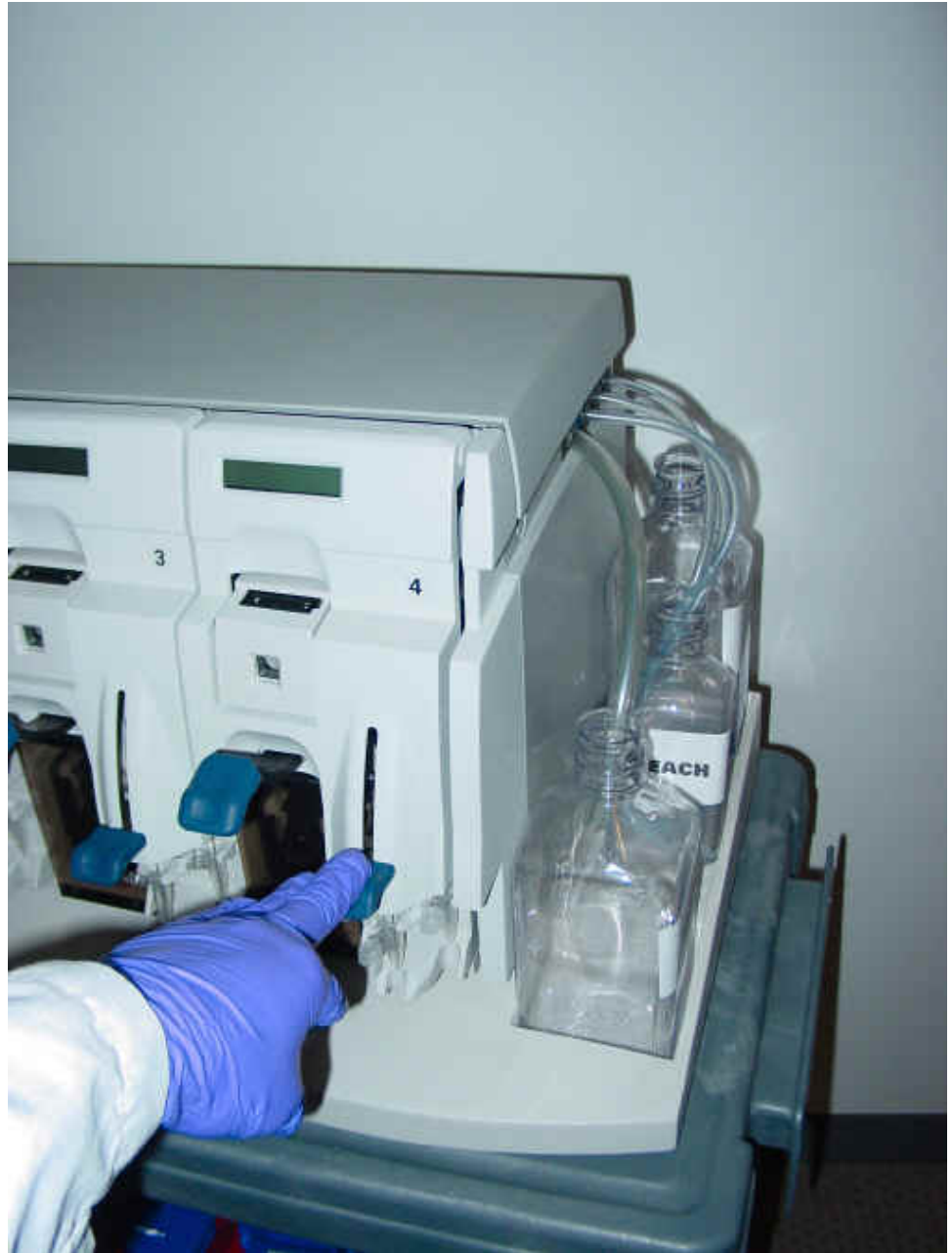
Figure 32 Press down on the needle levers to start the bleach protocol.
