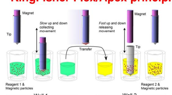
Inverse magnetic bead processing. Magnetic rods covered with tips are slowly moved up and down in bead suspension to collect the beads (well 1) Beads are transferred to the next plate where the beads are released in the reagent by tip mixing in the solution (well 2).
