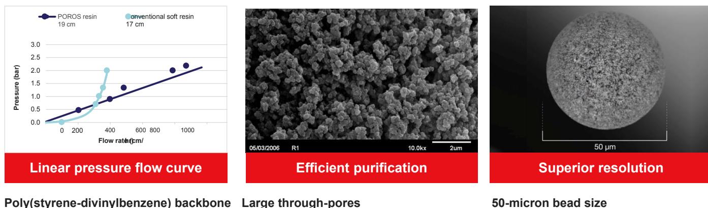
Figure 2. Key features of the POROS bead.
