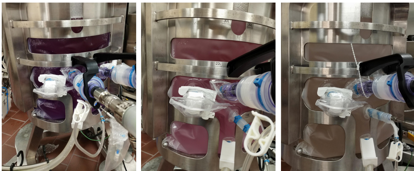
Figure 2. An anaerobic culture in the 50 L HyPerforma S.U.B. just after filtration (left), just after addition of hot L-cysteine (center), and just prior to inoculation with redox reading of about -275 mV (right).
