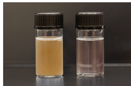
Before and after using Thermo Scientific™ Harvest RC Chromatographic Clarifier: turbidity reduction in a single stage
