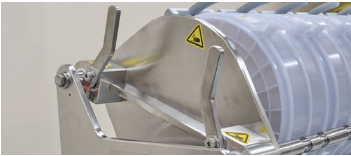
Two-handle locking mechanism
