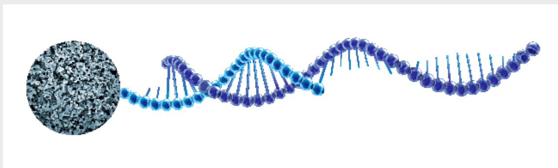
Schematic of Thermo Scientific™ POROS™ Oligo (dT)25 affinity resin, consisting of porous polymer beads coated with deoxythymine (dT) strands that can capture mRNA's poly-A tail. Image credit: Thermo Fisher Scientific
