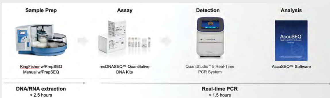
Figure 2: ResDNASEQ system integrates rapid sample preparation for nucleic acid extraction with a workflow for real-time quantitative polymerase chain reaction (PCR) analysis. Nucleic acid quantification can be used for rapid impurities and contaminant testing during regulatory quality control in biopharmaceutical production. Source: Thermo Fisher Scientific
