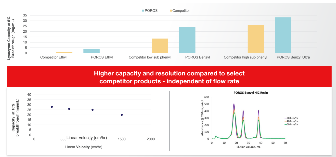
Figure 3. Comparison of key characteristics of POROS beads compared to select competitor products, highlighting higher capacity and resolution, independent of flow rate.
