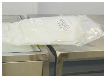
Figure 2.1. Smooth edges on an acceptable surface.
