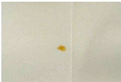
Figure 3.4. Gel particulate on BPC surface.
