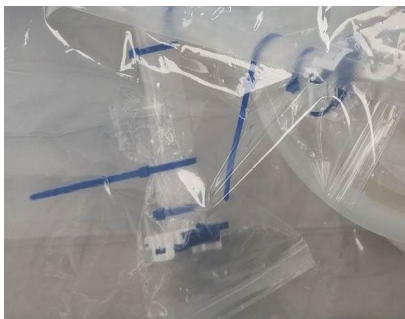
Figure 2.17. Tamper evident covers cable ties do not have tails snipped.
