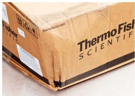
Figure 2.4. Worn box corner.
