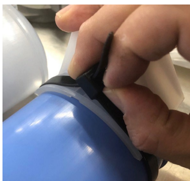
Figure 1.3. Pressing cable tie tab at the base of the filter.
