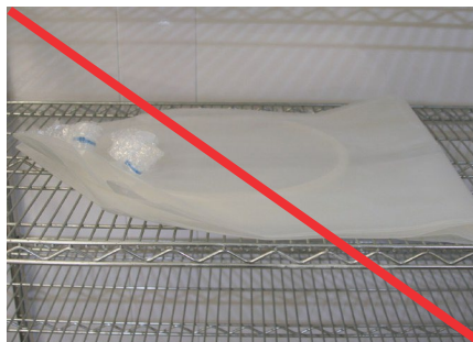
Figure 2.3. Wire rack as an unacceptable surface.
