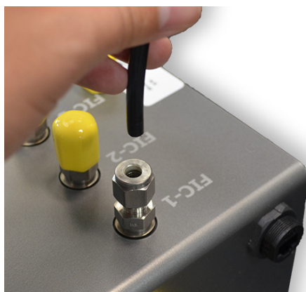
Figure 2.5. Inserting the pneumatic tubing into the TruFlow.
