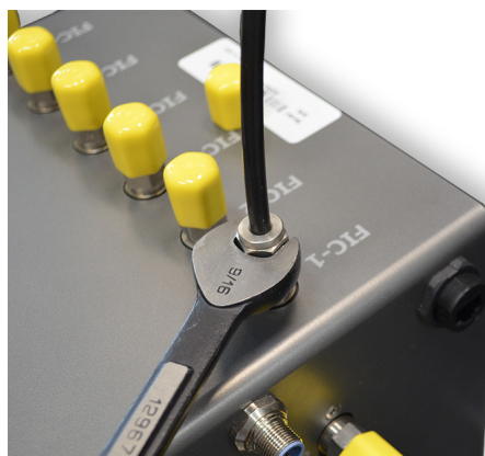
Figure 2.6. Using a 9/16 in. wrench to tighten the nut.
