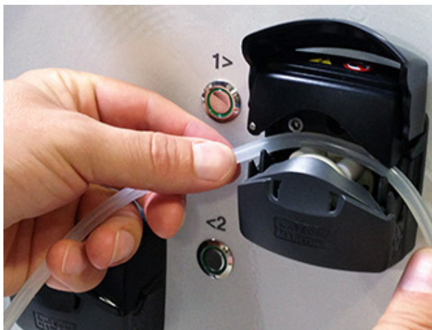
Figure 2.11. Installing pump tubing into pump.
