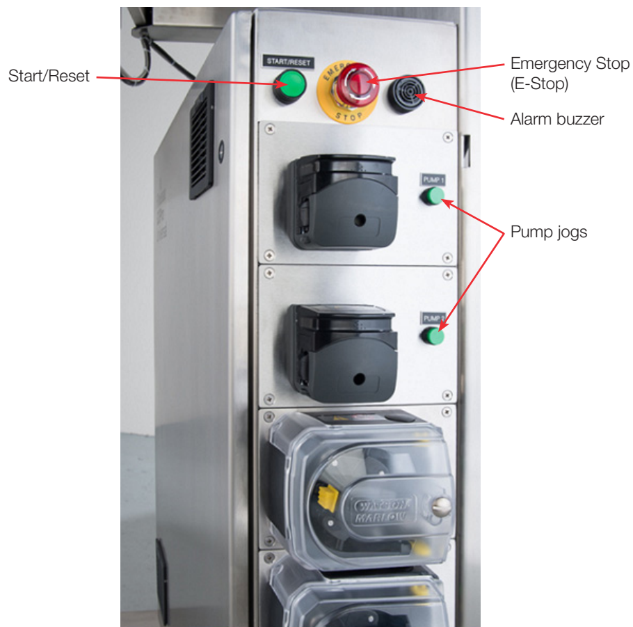
Figure 1.6. Upper half of the right side panel with pump heads.
