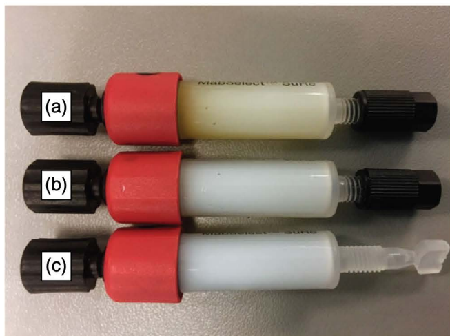
Figure 9. Picture of 1 mL MabSelect SuRe™ HiTrap Columns Post 100 PCC Cycles. Column (a) was loaded with depth filter clarified feed material, column (b) was loaded with FT-AEX clarified feed material, and column (c) is a fresh unused column.
