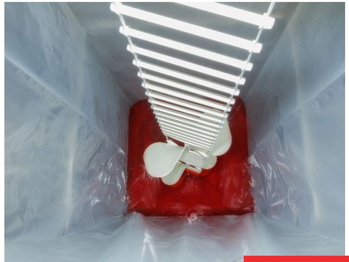
The flexible drive train includes multiple impellers that enable more PIV while still maintaining reasonable RPM and tip speeds.
