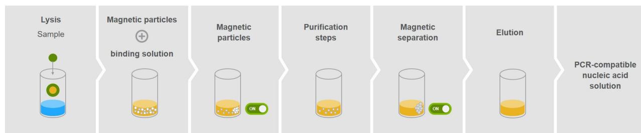
Figure 2. The PrepSEQ nucleic acid extraction workflow includes our proprietary magnetic particle and binding solution that not only supports high binding but complete elution of the purified sample.
