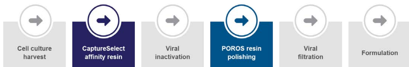
Figure 1. This workflow is depicting a typical downstream process for bio-therapeutics development. CaptureSelect and POROS resins can be used for both capture and polishing purification steps.
