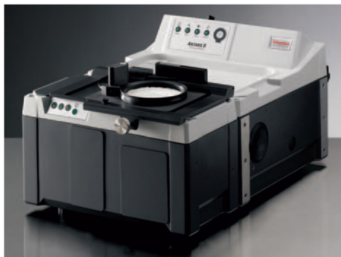
Figure 2. Antaris MDS with sample cup spinner.
