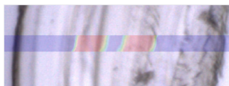
Video Image of the cross-section; FTIR image superimposed showing Nylon 6 layers.
