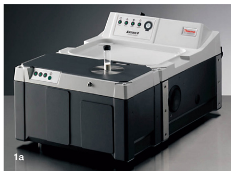
Figure 1. Antaris II MDS FT-NIR analyzer with integrating sphere (1a). The prepared samples were placed on top of the window over the integrating sphere, similar to what is shown in 1b, for the duration of the experiments.
