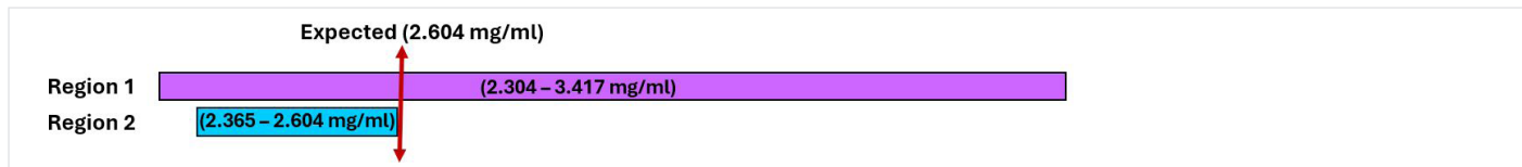
Figure 3. Range of values for the test solution (2.604 mg/ml) determined on the primary instrument and all 5 secondary instruments. Region 1 is 1432–592 cm -1 and Region 2 is 2960–2930 cm -1 .
