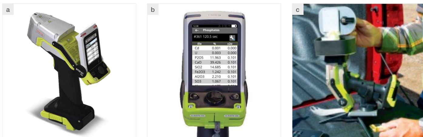
Figure 1. (a) Niton XL5 Plus analyzer; (b) Result of elemental analysis display for phosphate ore; (c) Sample analysis using the Thermo Scientific™ mini test stand.
