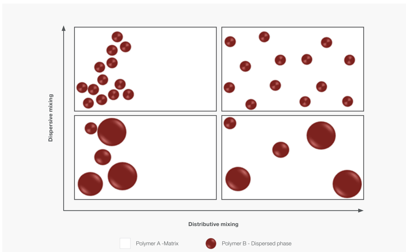
Figure 1. Schematic representation of morphology evolution in immiscible polymer blends (Polymer A + Polymer B) as a function of distributive and dispersive mixing intensity. Bottom left: limited distributive and dispersive mixing combined with poor interfacial stabilization results in droplet coalescence and the formation of large domains. Top left: insufficient distributive mixing leads to non-uniform spatial distribution of small domains within the matrix.
