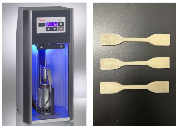
Figure 5. HAAKE MiniJet Pro Piston injection molding system and molded specimens.
