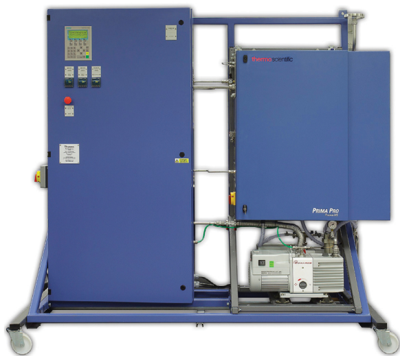
Figure 4. Prima PRO with VP variable pressure inlet and Thyson Technology sampling system
