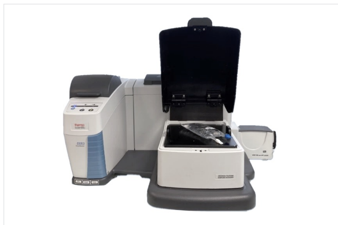
Figure 1. Infusion Bag placed in the DXR Universal Platform Sampling Accessory of the DXR3 SmartRaman spectrometer.
