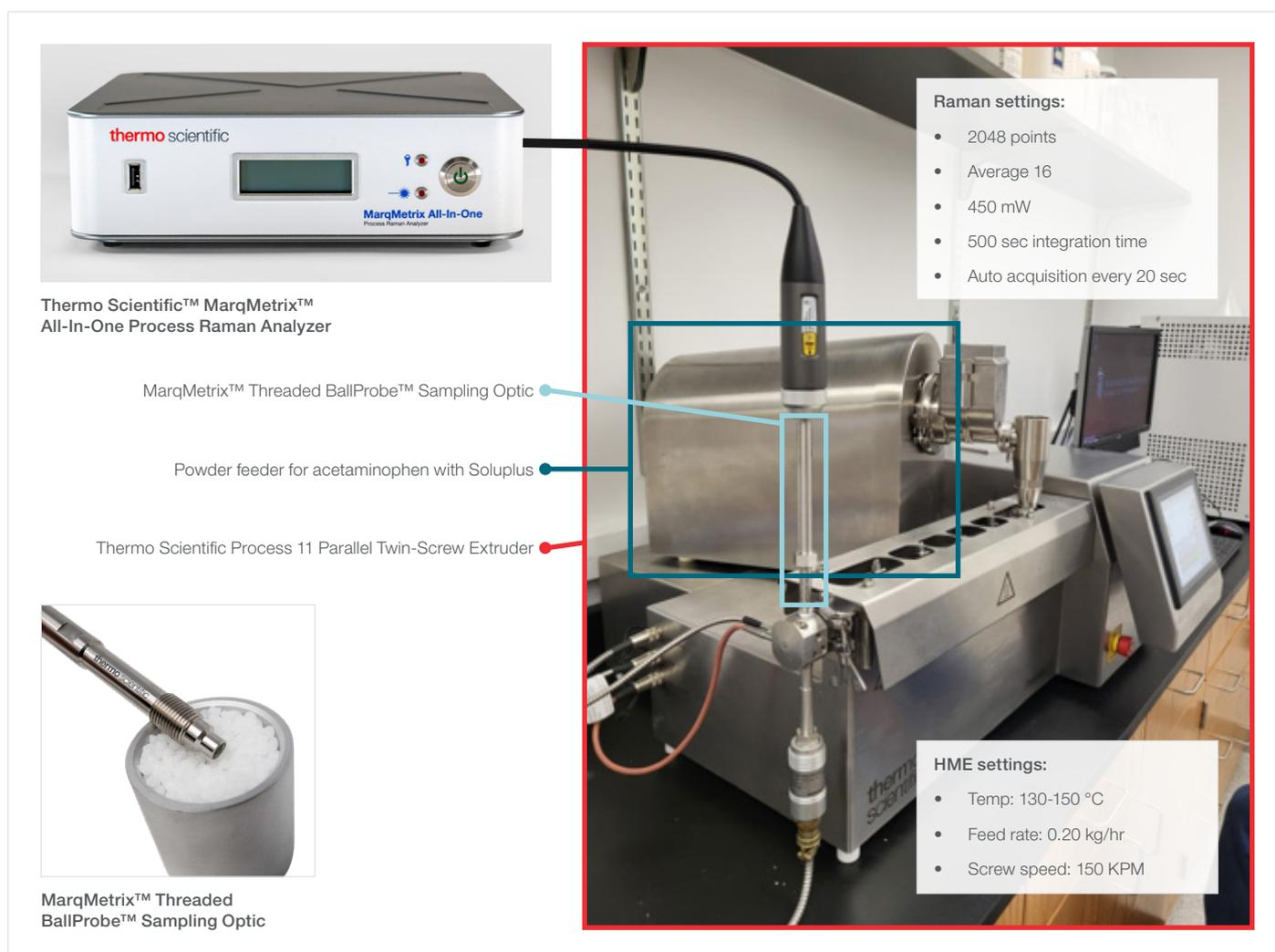
Figure 1. The Thermo Scientific MarqMetrix All-In-One Process Raman Analyzer and MarqMetrix Threaded BallProbe Sampling Optic, with the Thermo Scientific Pharma 11 Parallel Twin-Screw Extruder.
