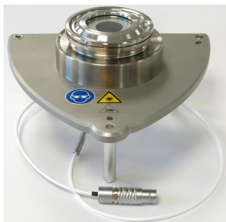
Figure 1. CM-OP-P module for UV measurements at ambient temperature.
