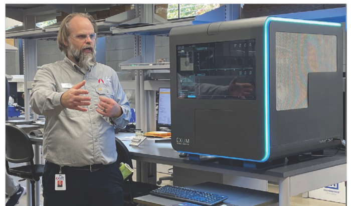
Figure 2: LIFT's Senior Metallurgist, Daniel Baker, explains how the MASSBOX LALI-TOF-MS operates as it analyzes a set of aluminum powder samples.
