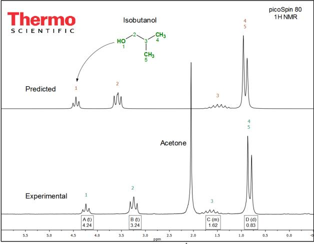
**Figure 5.** Full experimental (bottom) and predicted (top) <sup>1</sup>H NMR (82 MHz) spectrum of isobutanol in acetone (50:50 v/v).
