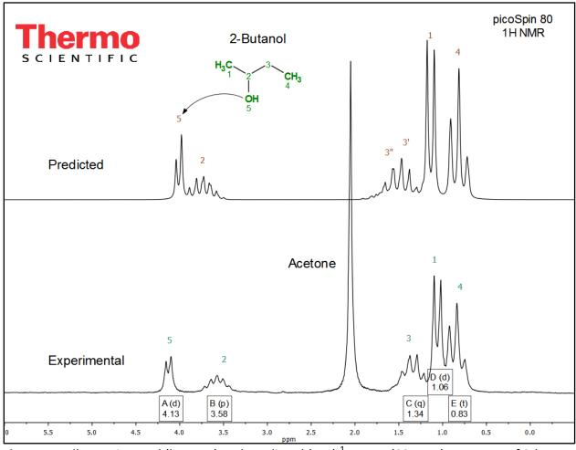
**Figure 4.** Full experimental (bottom) and predicted (top) <sup>1</sup>H NMR (82 MHz) spectrum of 2-butanol in acetone (50:50 v/v).
