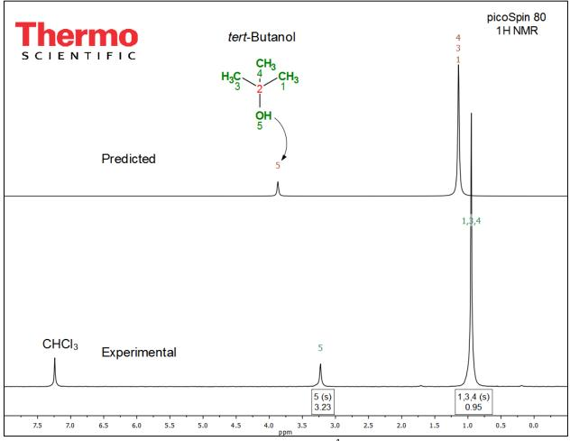
**Figure 6.** Full experimental (bottom) and predicted (top)  $^{1}$ H NMR (82 MHz) spectrum of *tert*-butanol in CHCl<sub>3</sub> (50:50 v/v).
