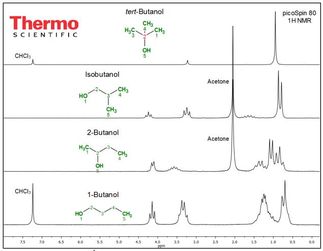
**Figure 1.** Full experimental <sup>1</sup>H NMR (82 MHz) spectra of, from top to bottom, *tert*-butanol, isobutanol, 2-butanol and 1-butanol.
