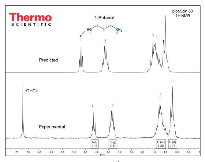
**Figure 3.** Full experimental (bottom) and predicted (top)  $^{1}$ H NMR (82 MHz) spectrum of 1-butanol in CHCl3 (50:50 v/v).
