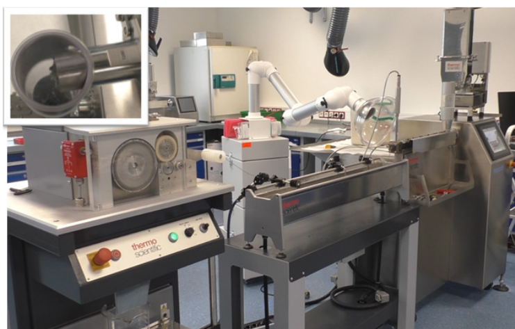
Figure 2. Process 16 extruder, water bath, pelletizer, filtration die, and rapid filter-insert exchange.
