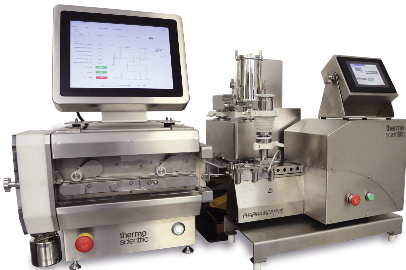
Figure 9. Standalone compounder and calibrated take-off / cutting device.
