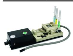
For controlled reactant mixing with applications in reactions with fast kinetics, this accessory allows a spectrometer to be used for following reactions that are at least a thousand times faster than those accessible manually.
