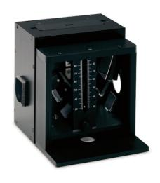
Measure film thickness or reflective properties from coatings at various angles from as low as 8 degrees to as high as 80 degrees. Accessory includes an alignment mirror that can also be used for baseline measurements.
