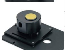
An SRA is specifically designed for use with reflective materials when measuring specular reflectance at a particular fixed angle.
