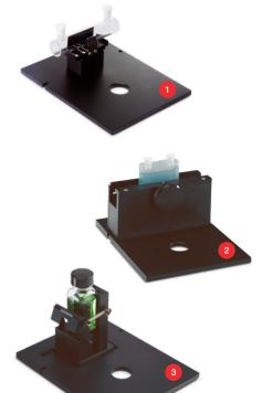
Different cell holders accommodate various sizes and shapes of rectangular, cylindrical, and test tube cells.
