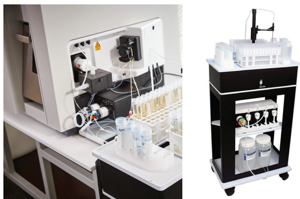
Figure 2. prep FAST auto-dilution system connected to the iCAP RQ ICP-MS (left). ESI SC-2DX autosampler (right).
