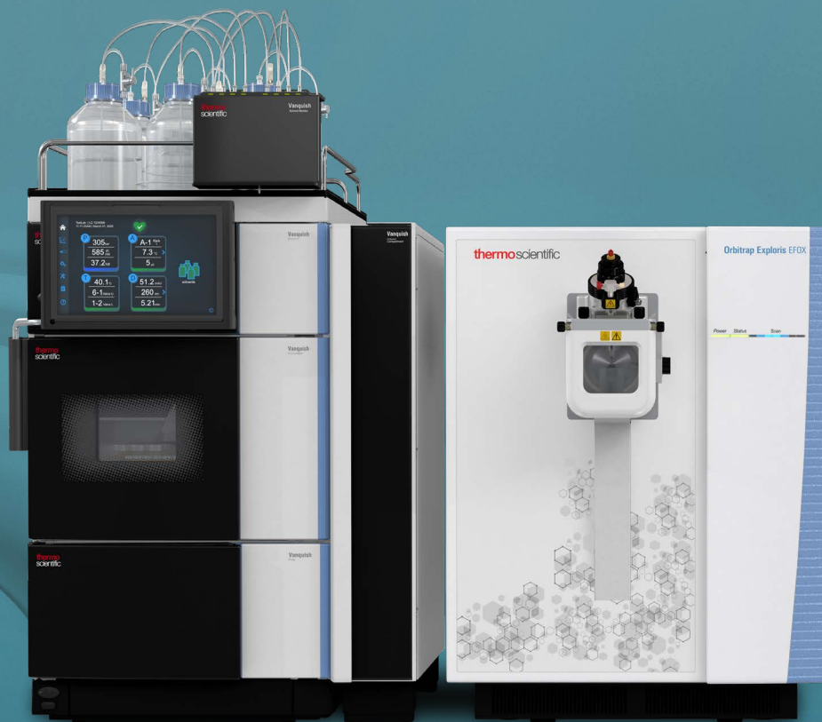
The Orbitrap Exploris EFOX Mass Detector coupled to the Thermo Scientific™ Vanquish™ Flex Duo dual channel system delivers built-for-purpose mass monitoring.
