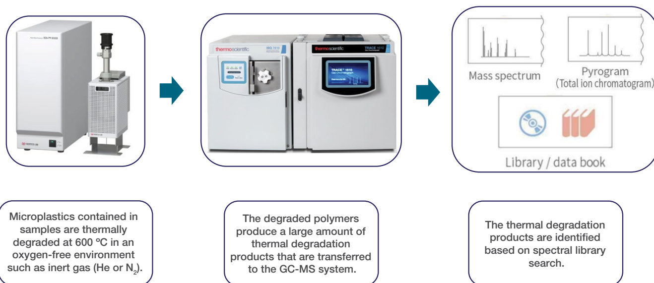
Figure 1. Schematic of Py-GC-MS workflow
