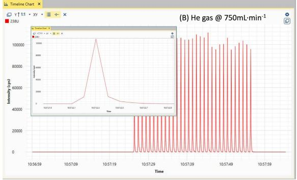
Figure 4. Comparison of washout time and peak shape between two different helium gas flow rates.
