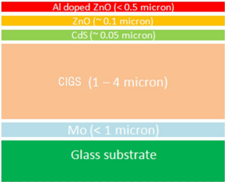
Figure 3: Typical CIGS multilayer
