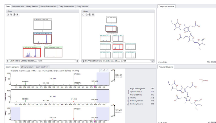
Figure 8: An example of substructure ID through MS n search matching portions of an unknown against the library compound stercobilin.
