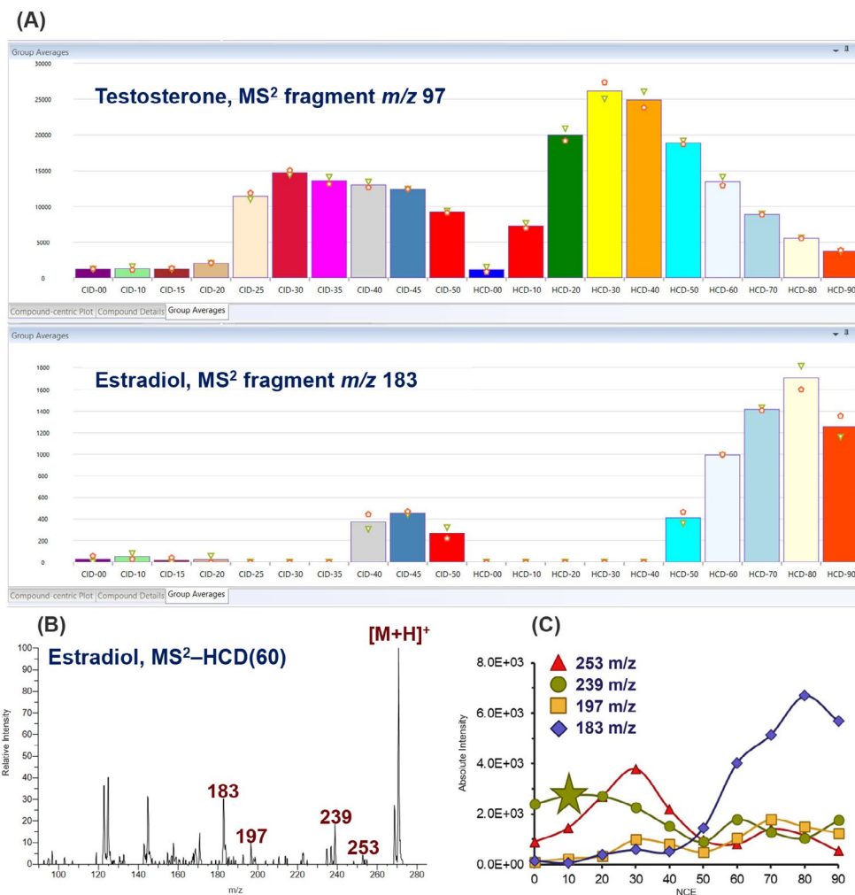
Figure 3. The determination of the optimal NCEs for steroids in CID and HCD MS 2 scan events in TraceFinder software using (A) testosterone fragment ion m/z 97 and estradiol fragment m/z 183 as examples; (B) MS 2 -HCD spectrum of partially fragmented estradiol precursor ion; (C) overlaid breakdown curves of estradiol MS 2 -HCD fragment intensities. The potential MS 3 candidates for estradiol are highlighted with an asterisk.
