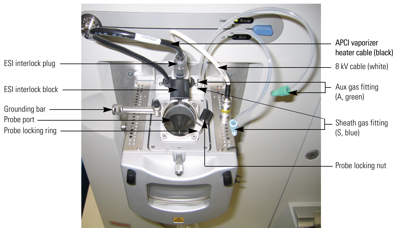
Figure 6. Ion Max ion source housing, no probe present
