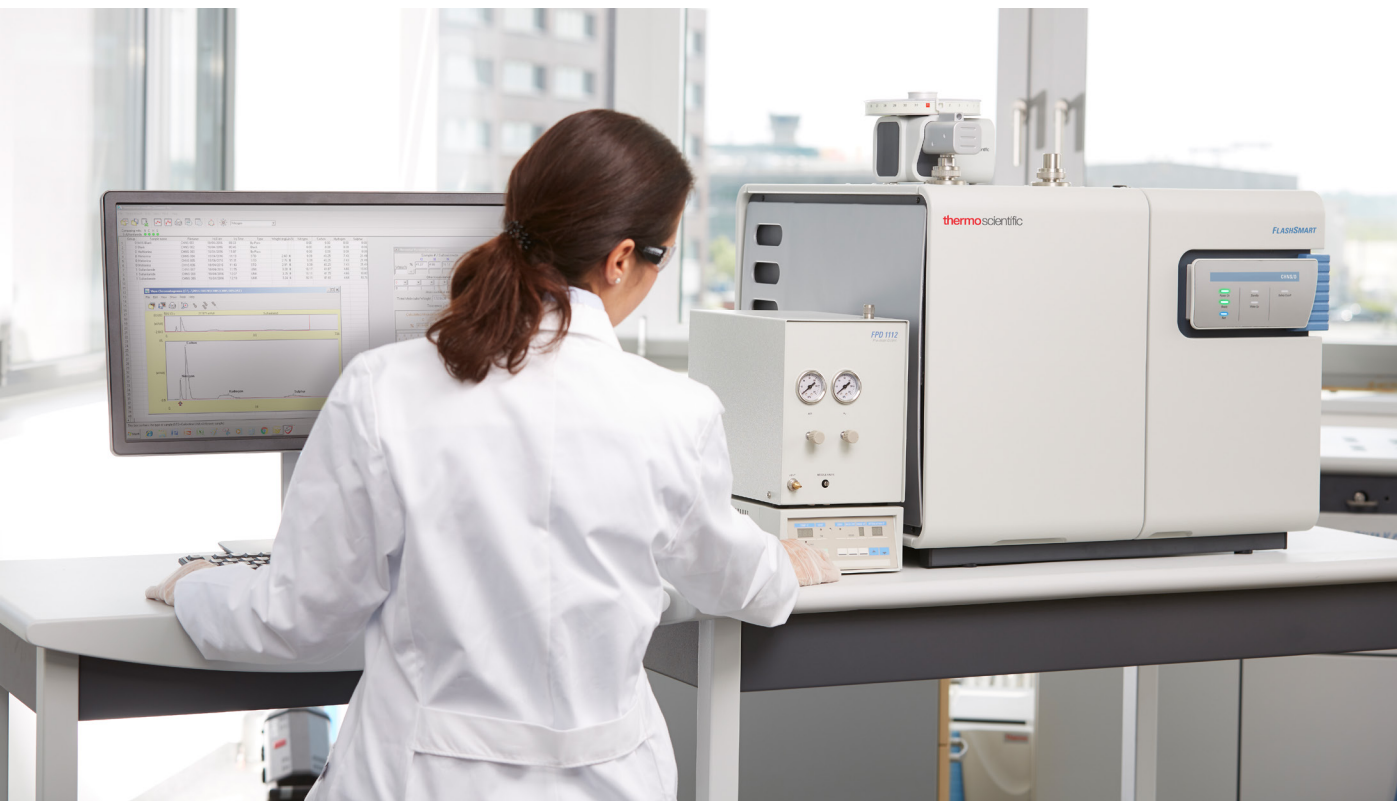
Figure 5. Thermo Scientific FlashSmart EA coupled with FPD Detector.
