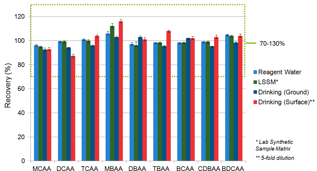
Figure 7. Precision and accuracy for haloacetic acid analysis in different water samples.
