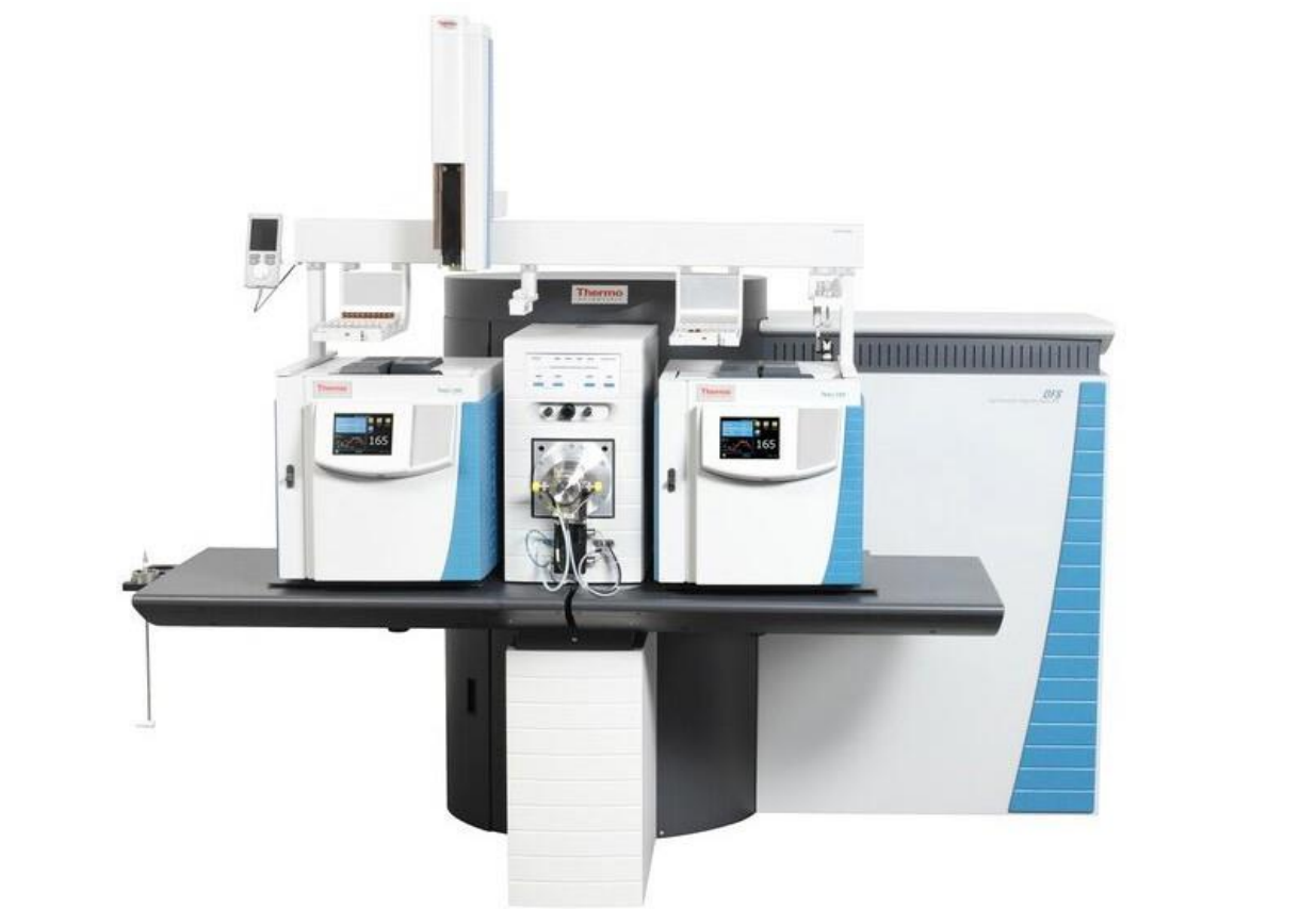
Figure 2. Thermo Scientific™ DFS™ Magnetic Sector GC-HRMS System
