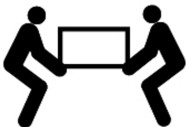
Figure 2-1. Lifting the centrifuge at both sides.
