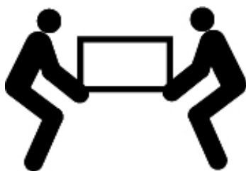
Figure 2-1. Lifting the centrifuge at both sides.
