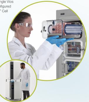
**1-21 % or 5-90 %** oxygen control ranges available in Tri-Gas configured Vios iDx CO<sub>2</sub> incubators. Simulate hypoxic (1-21 %) or hyperoxic (5-90 %) conditions for optimal growth of cells.
