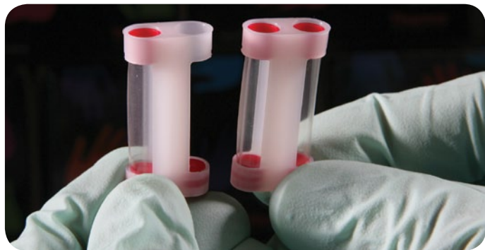
Figure 4. The different wells allow a choice of the size best suited for the specific experimental design. The plate and lid are made of high-grade reusable PTFE. The lid snaps onto the base plate and holds and suspends the disposable dialysis inserts in the wells to expose samples to a common dialysis matrix. RED Device Insert pictured on left and Competition RED Device Insert pictured on right.
