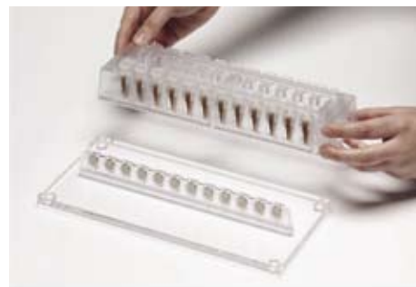
Figure 5—Process 24 samples at a time using the MagnaRack™ Magnetic Rack. The ChargeSwitch® gDNA Mini Bacteria Kit works well with the MagnaRack™ Magnetic Rack, which has precisely aligned neodymium magnets that enable processing of up to 24 microcentrifuge tubes in a variety of magnetic bead-based separations.
