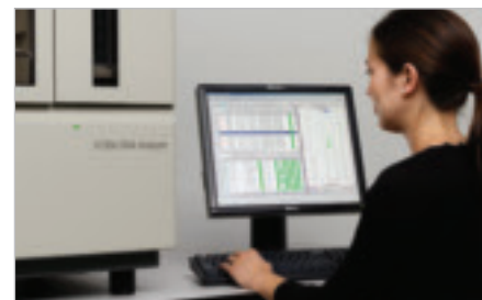
Figure 2. The SNPLex system offers an integrated solution including CE detection, data collection, and automated genotype calling.
