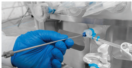
Figure 8. S.U.B. temperature sample port.
